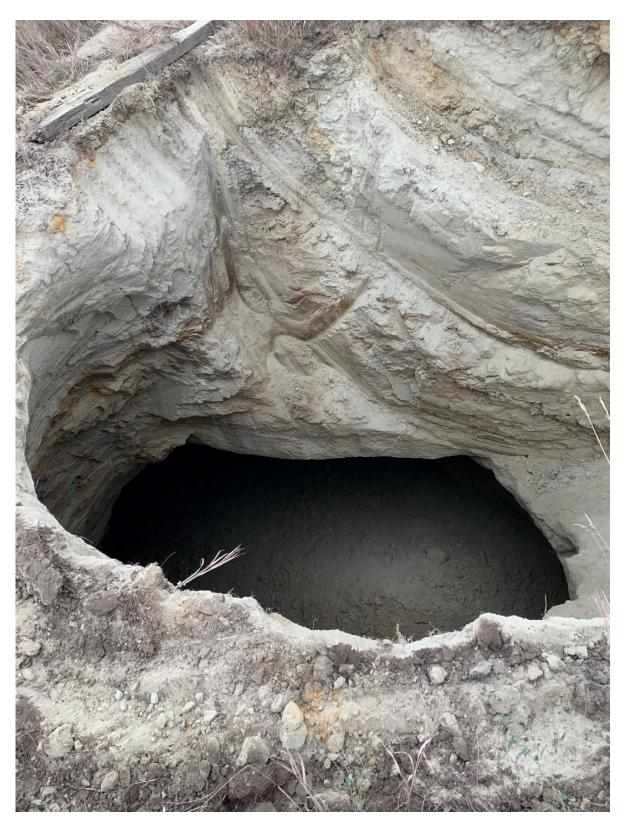
**Figure 8:** The same sinkhole was approximately 10 feet wide and measured 27 feet deep after the contractor removed the topsoil and subsoil.
